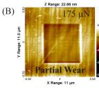
Depending on the applied load, different levels of wear can be observed.
